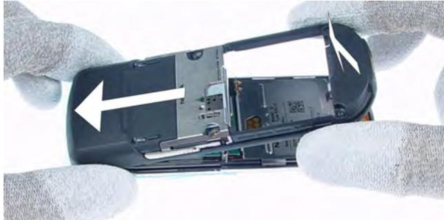
Remove the **B-cover** by shifting it carefully and as shown in the picture below. Mind the sharp contact springs.
