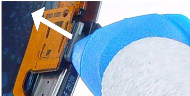
Carefully lever out the **camera module** with the SRT-6.
