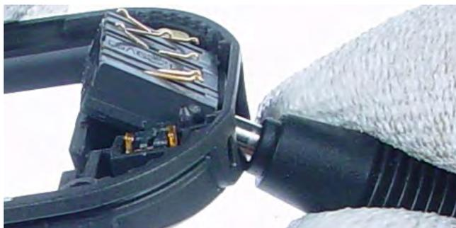
Use the **DC** plug to remove the system connector. Ensure that no adhesive remains.
