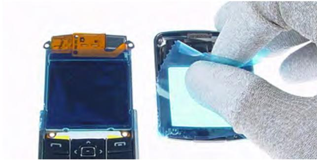
Protect the inner side window and now bared LCD with plastic film.
