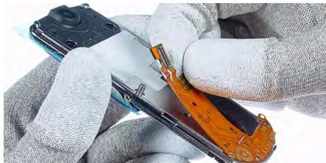
Peel off the **bottom flex** carefully.
