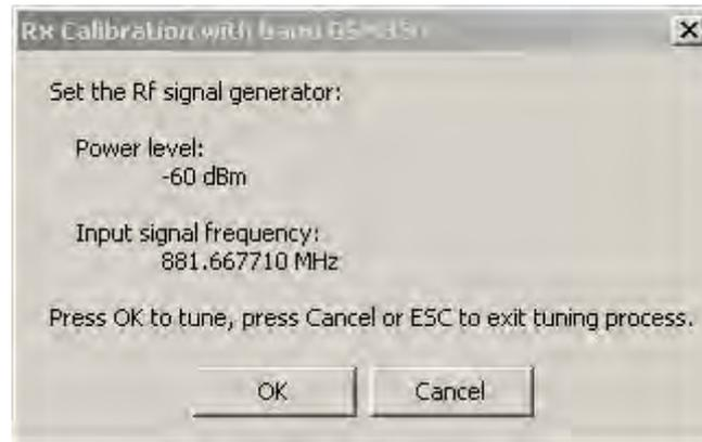
Figure 102 RX calibration with band EGSM900 (Example)
