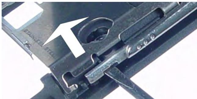
Unlock and remove the **SIM retainer**.
