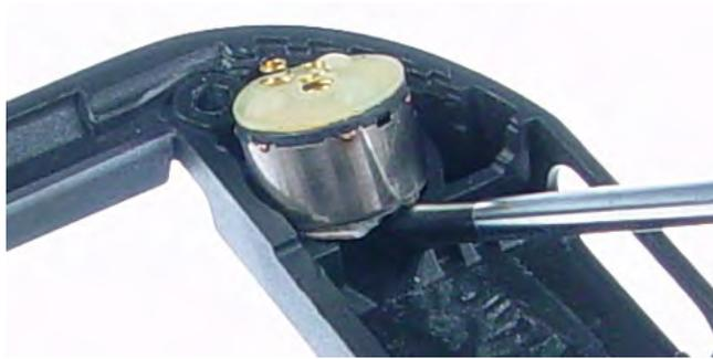
Lever out the **vibra motor** with a slotted screwdriver. Ensure that no adhesive remains.
